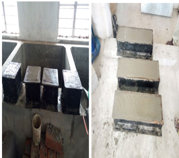
Fig. 4. Casting of the concrete.
