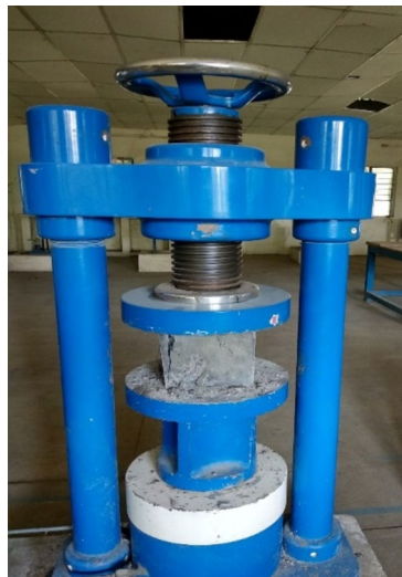
Fig. 7. Compressive strength test setup.
