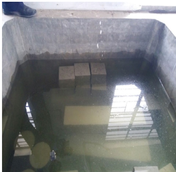
Fig. 5. Curing in progress.
