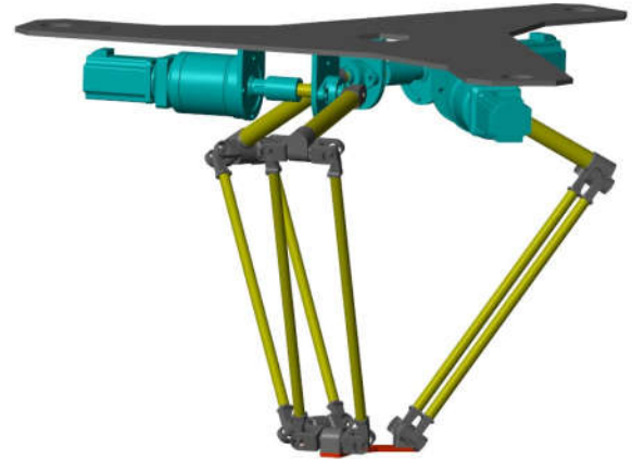
Fig. 2: Delta robot structure in Simscape.
