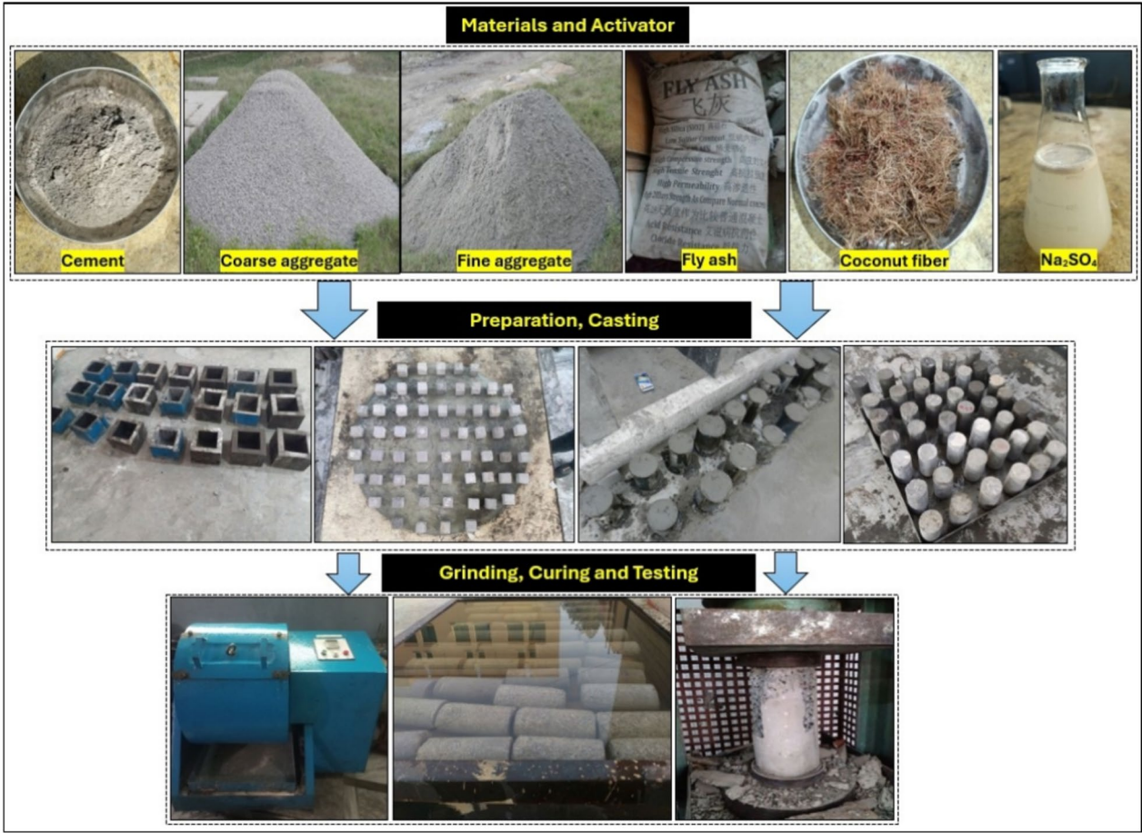
Fig. 1. The materials used, preparation, casting, grinding, curing and testing of this study.
