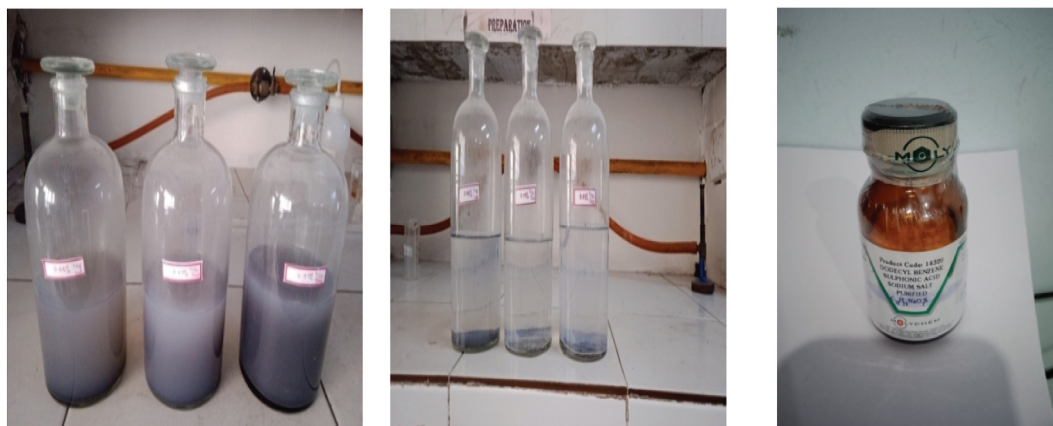
Figure 5. Various concentrations of the nanofluids prepared (0.01%, 0.03% and 0.05%) a) after 1-day b). 0.01% ,0.03% and 0.05% (after 60 days) c) Surfactant (SDBS).
