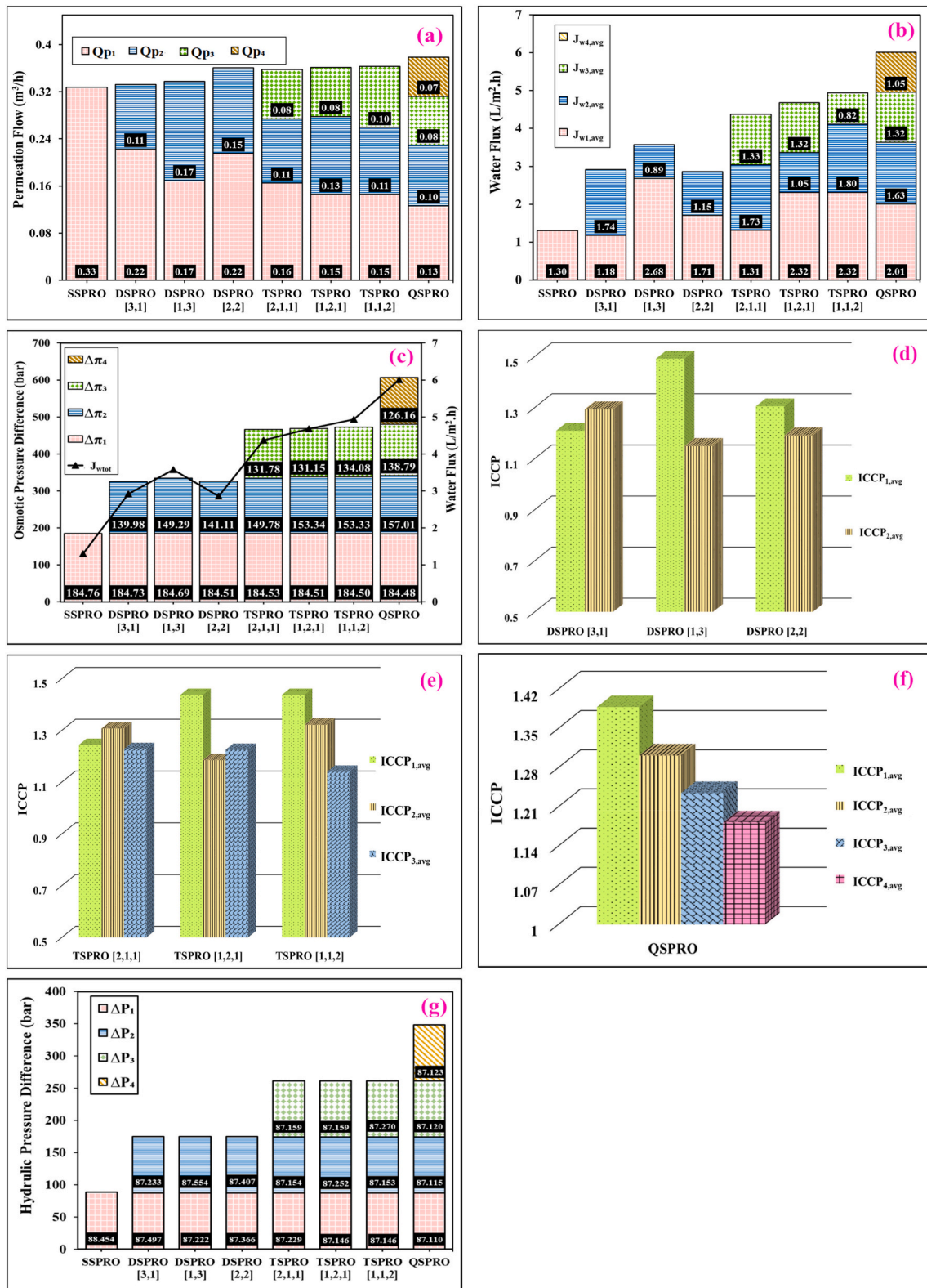
Fig. 3. (a) The permeation flow in the first, second, third, and fourth PRO stages ( Q_{p1} , Q_{p2} , Q_{p3} , and Q_{p4} , respectively) in the single-stage PRO (SSPRO) and the multistage PRO scenarios, (b) the average water flux in the first, second, third, and fourth PRO stages ( J_{w1,avg} , J_{w2,avg} , J_{w3,avg} , and J_{w4,avg} , respectively) in the single-stage PRO (SSPRO) and the multistage PRO scenarios, (c) the total water flux ( J_{w,tot} ) and the osmotic pressure difference in the first, second, third, and fourth PRO stages ( \Delta\pi_1 , \Delta\pi_2 , \Delta\pi_3 , and \Delta\pi_4 , respectively) of the SSPRO and the multistage PRO scenarios, (d) the average internal concentration polarization in the first and the second PRO stages ( ICCP_{1,avg} and ICCP_{2,avg} , respectively) in the dual-stage PRO (DSPRO) scenarios, (e) the average internal concentration polarization in the first, the second, and the third PRO stages ( ICCP_{1,avg} , ICCP_{2,avg} , and ICCP_{3,avg} , respectively) in the ternary-stage PRO (TSPRO) scenarios, (f) the average internal concentration polarization in the first, the second, the third, and the fourth PRO stages ( ICCP_{1,avg} , ICCP_{2,avg} , ICCP_{3,avg} , and ICCP_{4,avg} , respectively) in the quaternary-stage PRO (QSPRO) scenario, and (g) the hydraulic pressure difference in the first, second, third, and fourth PRO stages ( \Delta P_1 , \Delta P_2 , \Delta P_3 , and \Delta P_4 , respectively) of the SSPRO and the multistage PRO scenarios.
