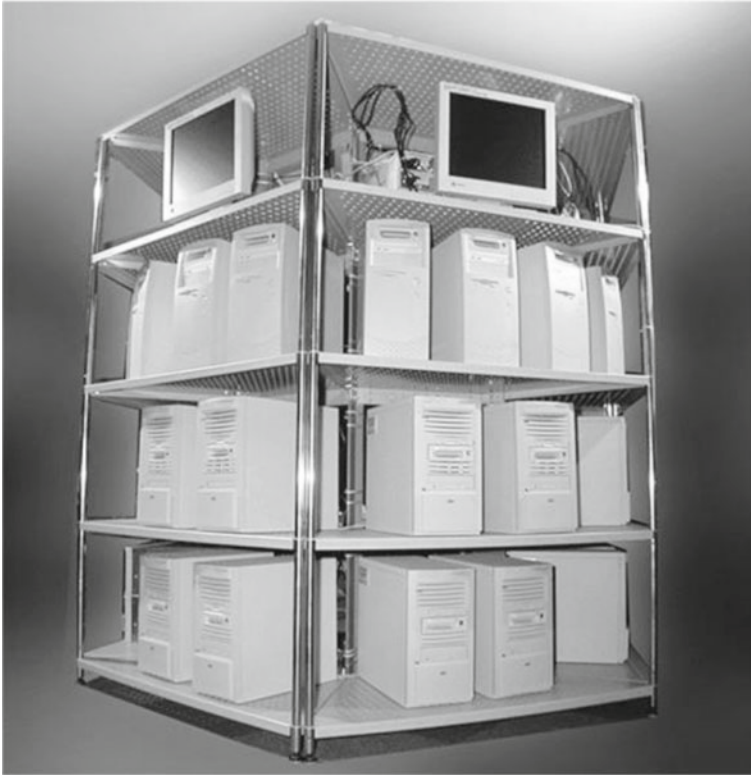
Fig. 8.9 Heterogeneous cluster consisting of 16 x86 CPUs and 16 DEC Alpha CPUs. This cluster was demonstrated at the SC'99 exhibition
