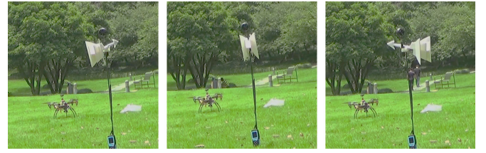
Fig. 7. The fully automatic realtime aerovane.
