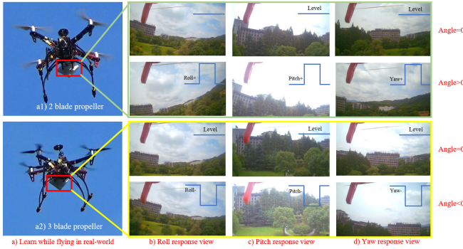
Fig. 10. The real-time snapshots of the UAV's periodic command steps response process under the condition of unknown power configuration in real-world.
