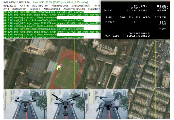
Fig. 3. Snapshot of SITL for quadcopter attitude controller adaptive learning. There are three main parameters [K_p, K_i, K_d] for a single channel. Previous research shows that the proportional term coefficient K_p is the primary influence. Therefore, in this paper, we give the initial values \mathbf{K}_i(0) and \mathbf{K}_d(0) of ZN adjustment in the SITL simulation environment and real test flight environment in advance, mainly for the \mathbf{K}_p term, which has more influence on stability.
