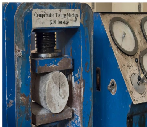
(c) Split tensile testing
