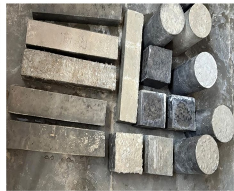
(f) Broken specimens 3
