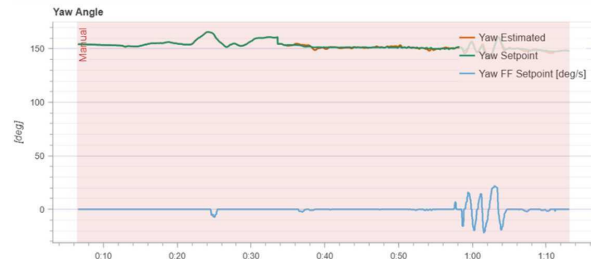
Fig. 9. Yaw angle of the UAV over time.
