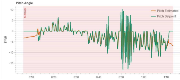
Fig. 8. Pitch angle of the UAV over time.
