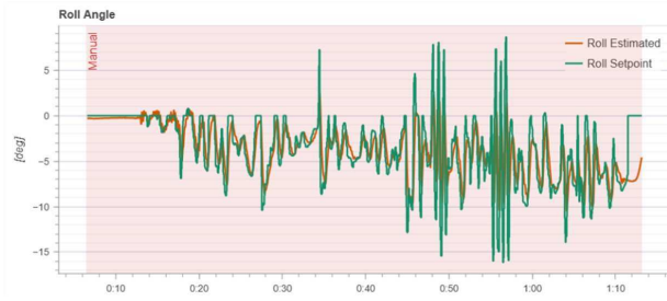
Fig. 7. Roll angle of the UAV over time.
