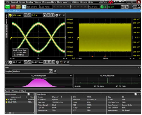
Fig. 8. Measured 56GHz clock pattern jitter.
